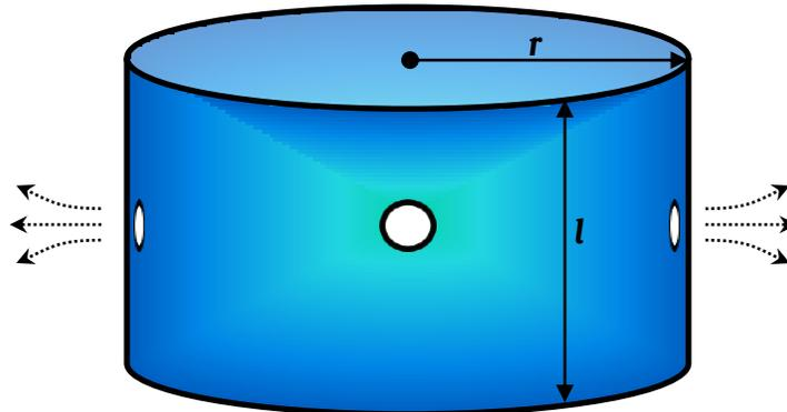
**Figure 1 – AV Bay Pressure Equalization**
