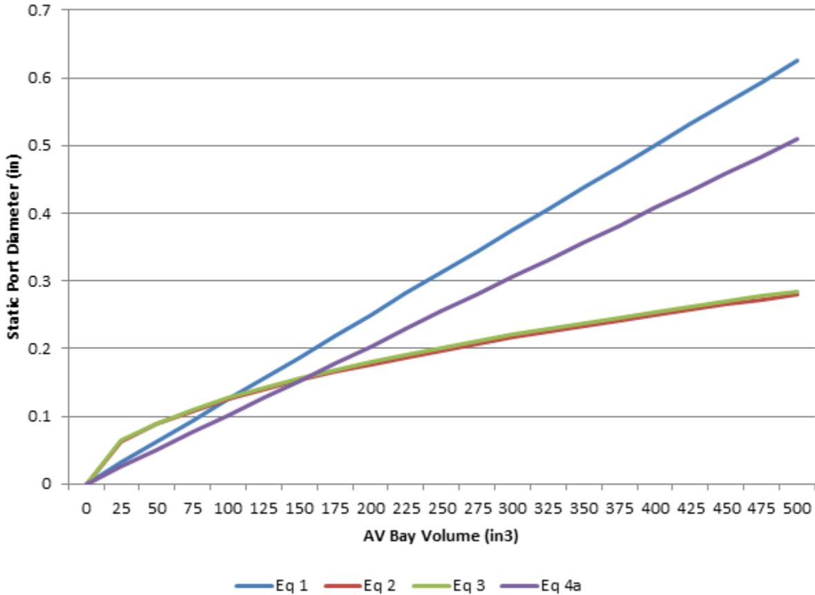
**Figure 3 – 4 Port Static Port Sizing**
