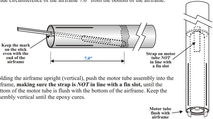
Holding the airframe upright (vertical), push the motor tube assembly into the airframe, **making sure the strap is NOT in line with a fin slot**, until the bottom of the motor tube is flush with the bottom of the airframe. Keep the assembly vertical until the epoxy cures.
