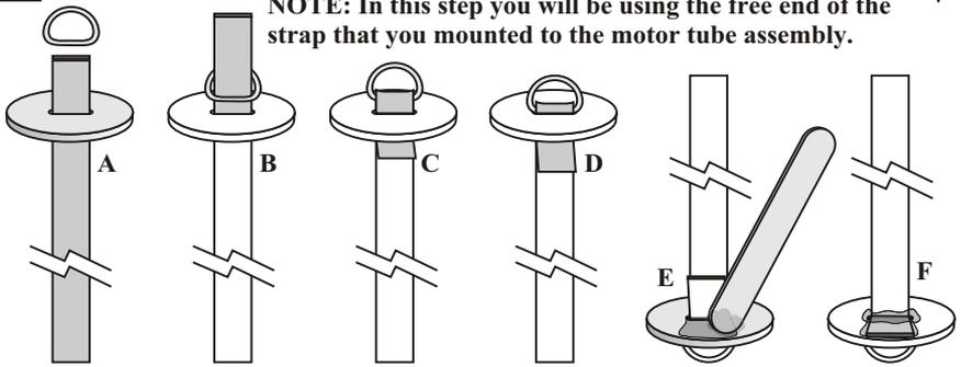
**A)** Pull the free end of the strap through the slot in the piston bulk plate.
