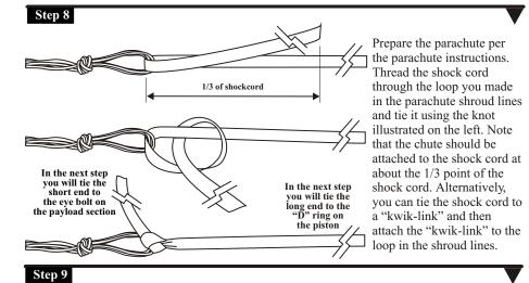
Thread the long end of the shock cord through the "D" ring and tie it using the knot illustrated below. Alternatively, you can tie the shock cord to a "kwik-link" and then attach the "kwik-link" to the "D" ring. Use the same knot to attach the other end of the shock cord to the eye bolt on the payload section.
