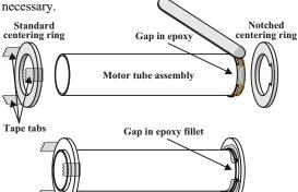
Spread a bead of epoxy around the circumference of the threaded adapter retainer leaving a 1" gap in the bead at the notch in the rib. Slip the notched centering ring over the threaded adapter retainer with the notch aligned with the gap in the epoxy bead. Be sure the notch in the ring remains clear of epoxy. Locate the ring against the rib and with the notches aligned. Allow the epoxy to set
