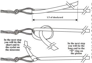
Prepare the parachute per the parachute instructions. Thread the shock cord through the loop you made in the parachute shroud lines and tie it using the knot illustrated on the left. Note that the chute should be attached to the shock cord at about the 1/3 point of the shock cord. Alternatively, you can tie the shock cord to a "kwik-link" and then attach the "kwik-link" to the loop in the shroud lines.
