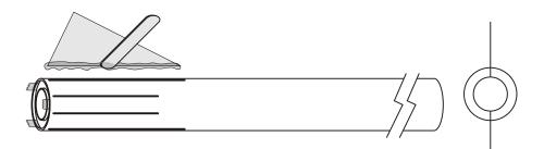
**D**) The four remaining slots are for the four small fins. Apply a bead of epoxy to the root edge of a fin. Push the fin through the slot in the airframe and against the motor mount tube. Make sure that the fin is perpendicular to the airframe. Use tape to hold the fin in position while the epoxy cures. Repeat this process for all fins.
