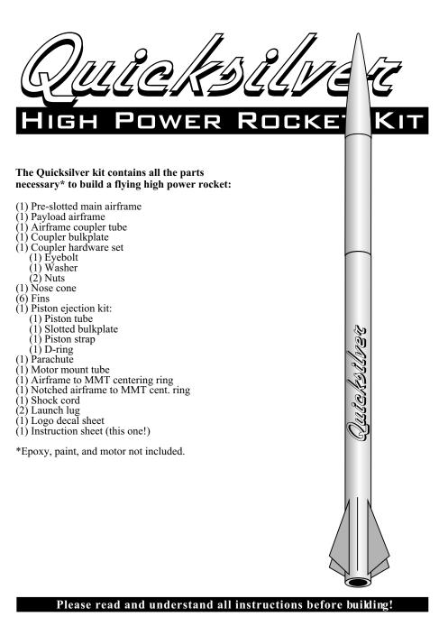
The center of pressure (CP) of this rocket is 41.6 inches from nose tip. After finishing your rocket, permanently mark the center of pressure on the airframe. After loading the rocket with a motor, make sure that the center of gravity (balancing point) is at least one body diameter forward of the center of pressure mark. The center of gravity can be moved forward by adding weight to the nose cone.
